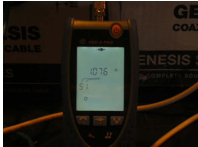
This Ideal VDV II Pro tester is connected to 1,076 feet of coax cable. (Source: David J. Engebretson)
