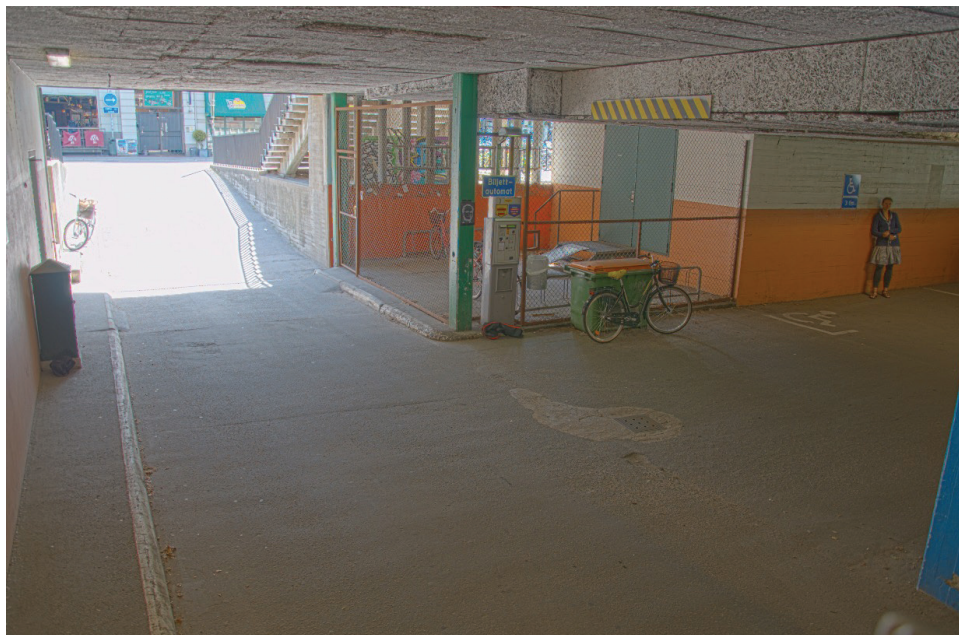
The same parking garage depicted through a WDR camera. Notice that the WDR camera clearly shows details both in the well-lit entrance and the dark shadows.
