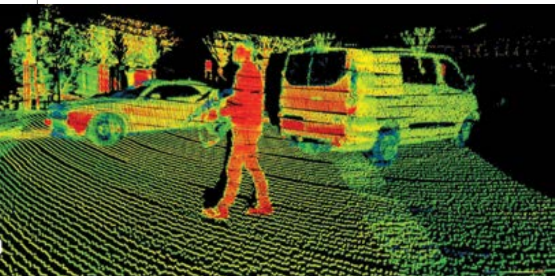
Raw LiDAR data of a human and vehicles
