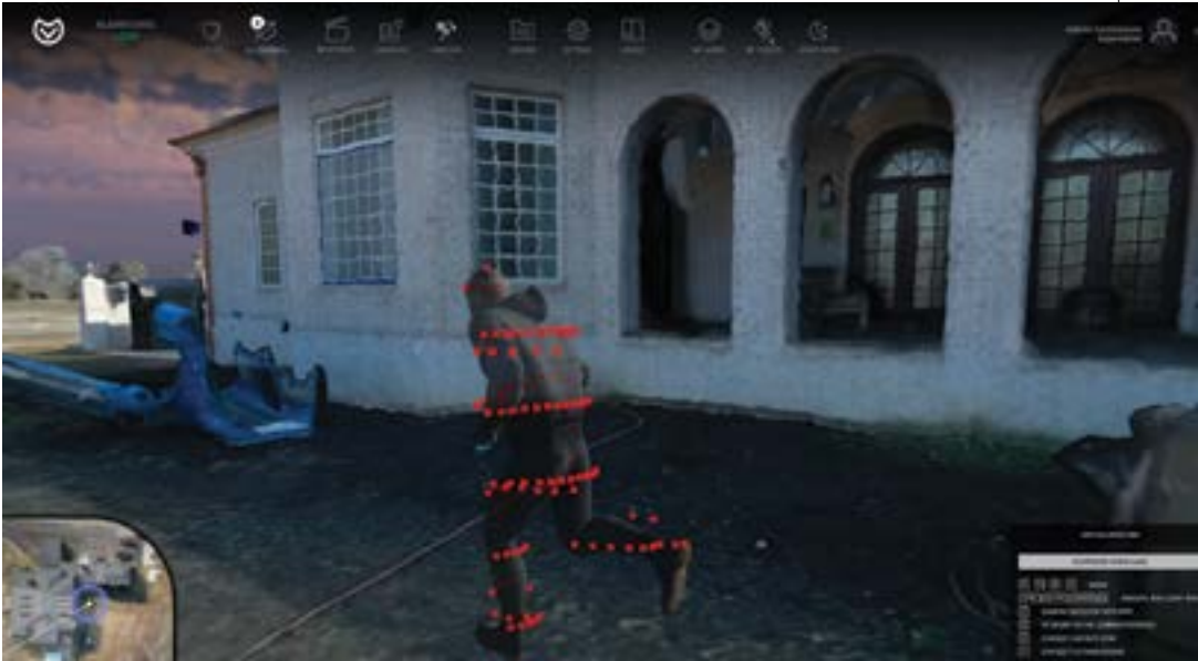
LiDAR detector locations being tested for effectiveness within the 3D map by moving a virtual intruder through the scene
