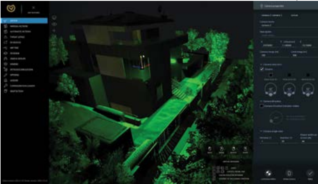
Security camera coverage and blind spots depicted in the 3DSCS using a green light source and shadows
