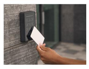
Physical access controls are another aspect of a security solution that can integrate seamlessly with some video management systems. Access controls ensure that only authorized personnel are allowed entrance to a site, to a particular building, or even within certain areas of a building, and during which hours of the day an individual has access.
